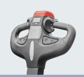
Simple and beautiful tiller designed to operate all functions easily even by one hand. Displayed turtle speed function applied to move slowly and helps to stack goods in narrow spaces
