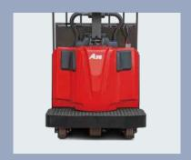
The roomy platform features low steps neights to reduce fatigue, and cushioned ean pads (Opt.) allow the operator to adjust stance throughout the shift, enhancing operator comfort
